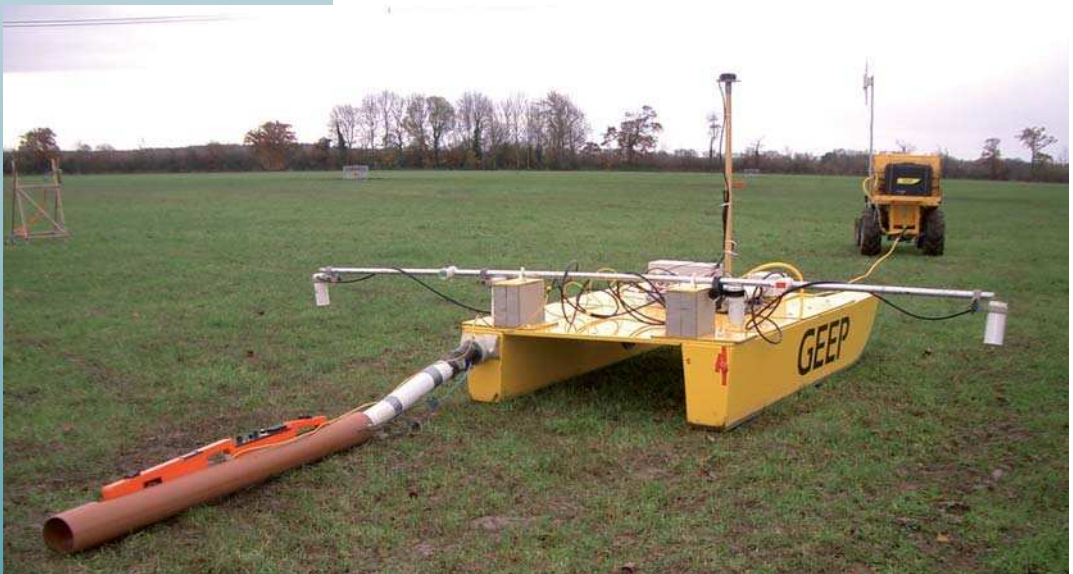
Figure 1: The GEEP towed mobile sensor platform with built-in GPS. (photograph courtesy of Ian Hill, University of Leicester).
